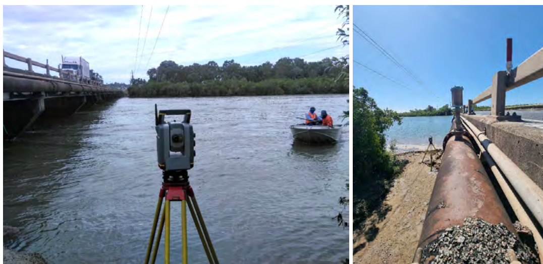
Figures 1 and 2: Surveying for renewal of the water main over Alligator Creek
