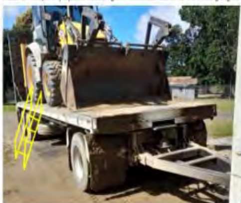
Photo 5. Example of proposed access/ egress: removable ladder for the existing dog trailers in the fleet.
