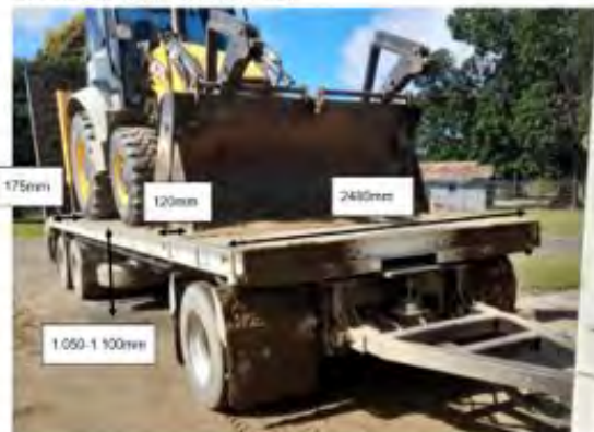
Photo 3 Backhoe trailer clearance / measurements
