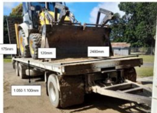
Photo 3 Backhoe trailer clearance / measurements
