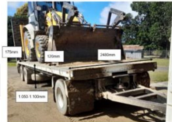
Photo 3 Backhoe trailer clearance / measurements
