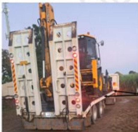
Photo 2 – Backhoe loaded- note lack of available space for operator to walk around plant on trailer deck.
