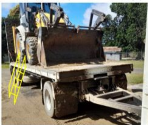
Photo 5. Example of proposed access/ egress- removable ladder for the existing dog trailers in the fleet
