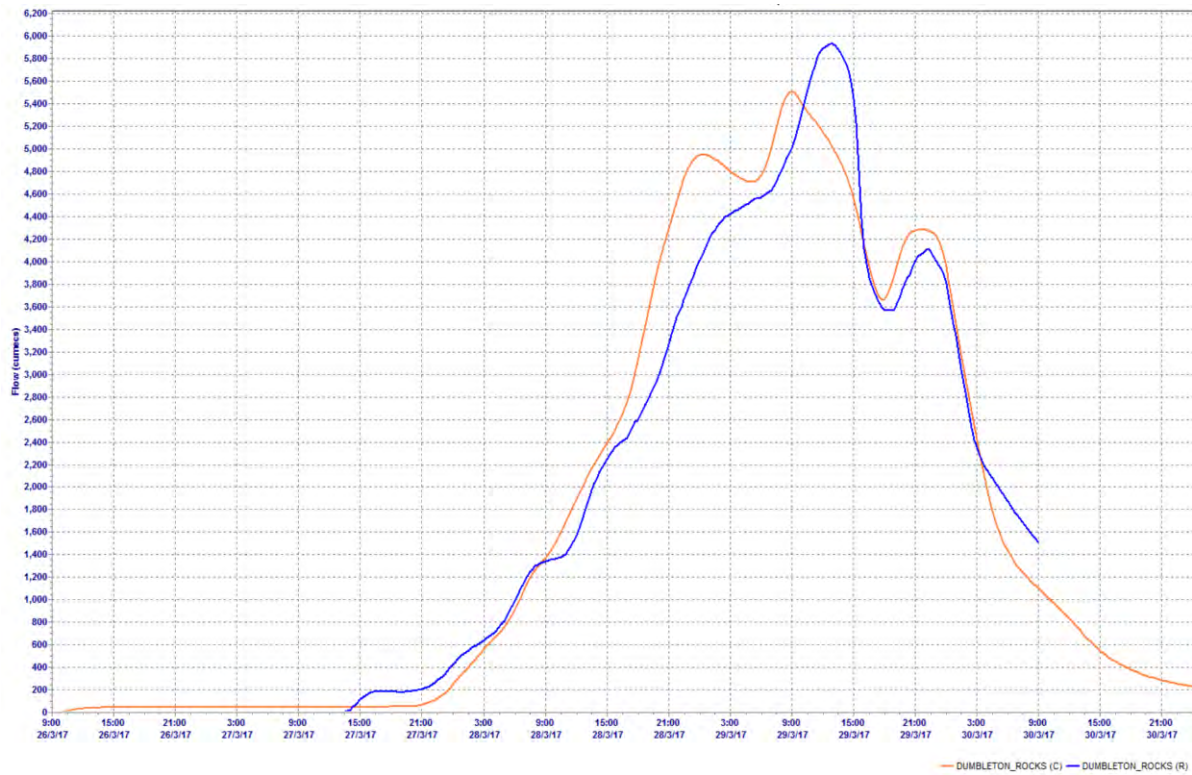
Figure 4.48 - Comparison of recorded and URBS model predicted discharges, Pioneer River at Dumbleton HW, March 2017 event
