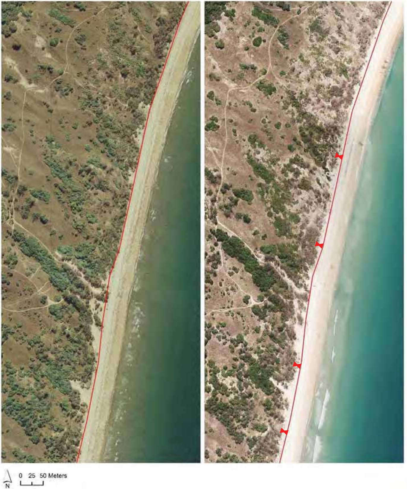
Figure 28: North Harbour Beach– aerial imagery 2009 (left) and 2015 (right) indicating shoreline recession in the order of 8–15m and up to 20m in some locations. Red line indicates approximate 2009 shoreline position.
