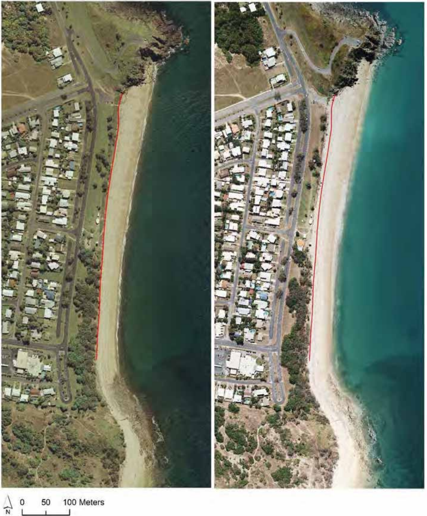
Figure 27: Lamberts Beach aerial imagery – 2009 (left) and 2015 (right) indicating recent shoreline retreat in the order of 5-15m. Red line indicates 2009 approximate shoreline position.
