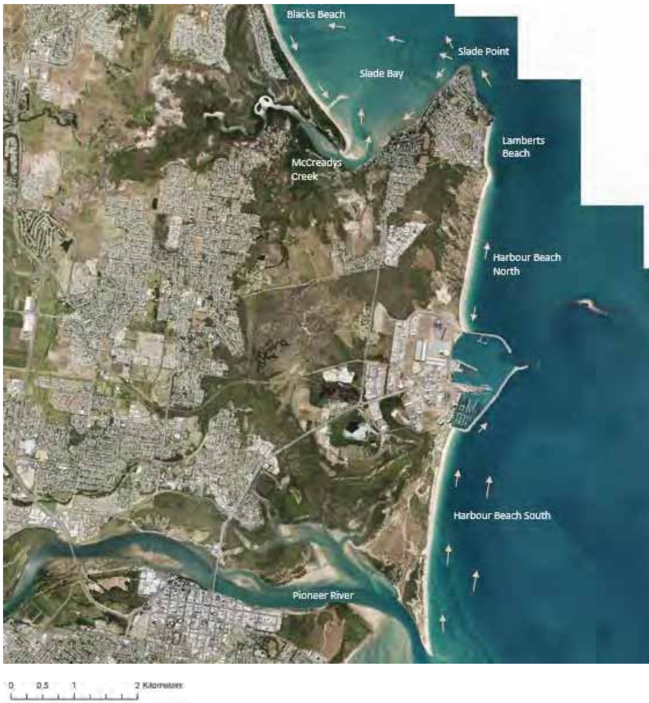
Figure 21: Mackay coastline aerial (DEHP 2015) - Harbour Beach South to Slade Bay – Indicative longshore sediment transport noted by arrows - after EPA (2004).
