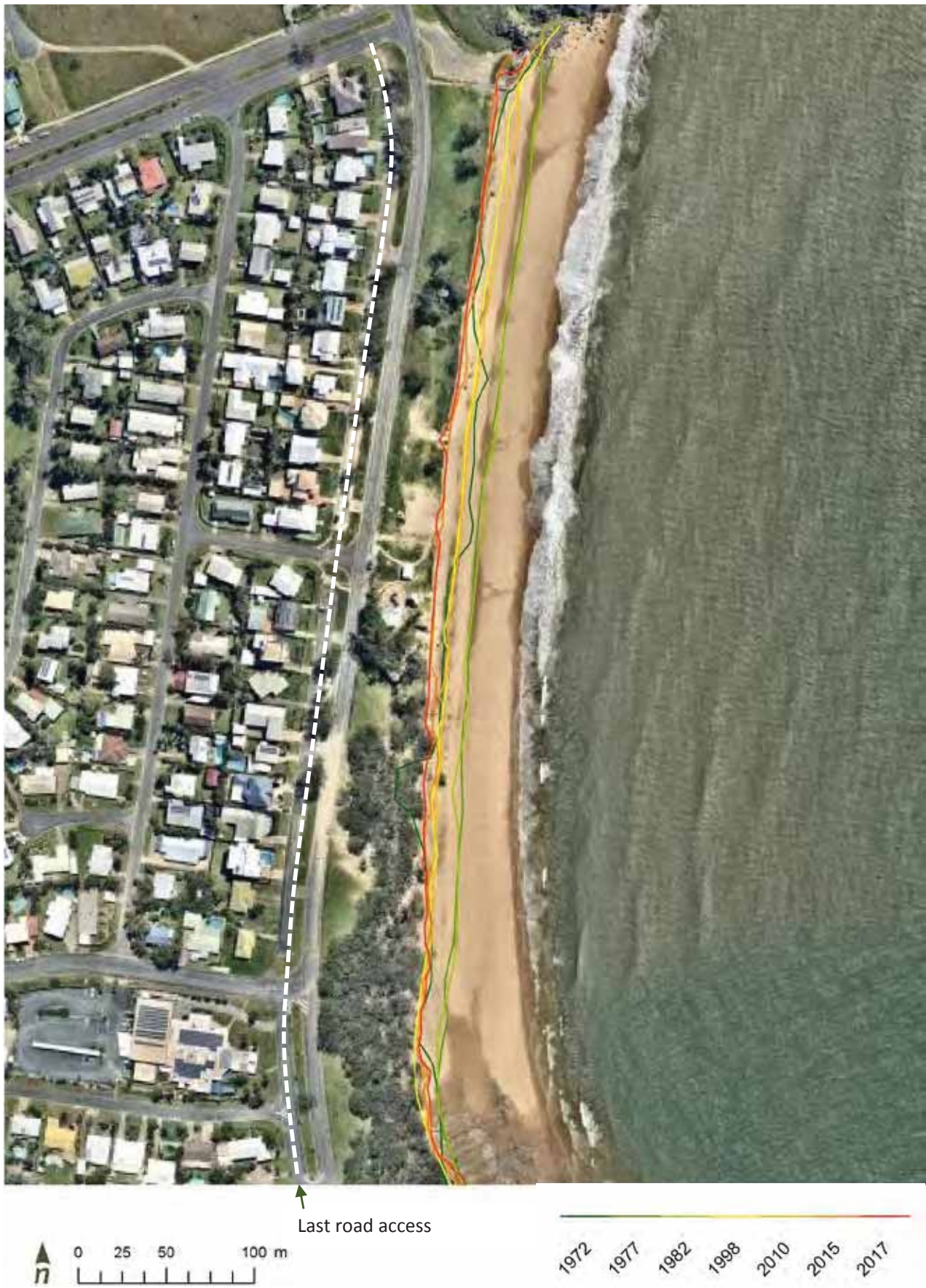
Figure 25: Comparison of indicative shoreline positions from 1972 to 2017. Note change reflects only the visible difference in the mature vegetation/scarp line from aerial imagery. Change does not reflect the volume of sediment lost from the toe of the scarp line and frontal dunes as observed on the ground in June 2017 inspections. The 1977 shoreline position represents the shoreline once development of the area was completed, and is the benchmark for assessing subsequent shoreline change and erosion rates. At the closest point, there is around 50m from the scarp line to the last road access.
